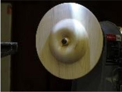
**Top Tip 3** - When reducing the thickness do a bit at a time working inwards to prevent flexing.
