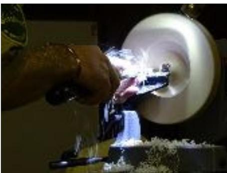
**Top Tip 2** - the bowl gouge is easier to control if the left hand grips under the tool rest and the right hand thumb carefully pushes the gouge.
