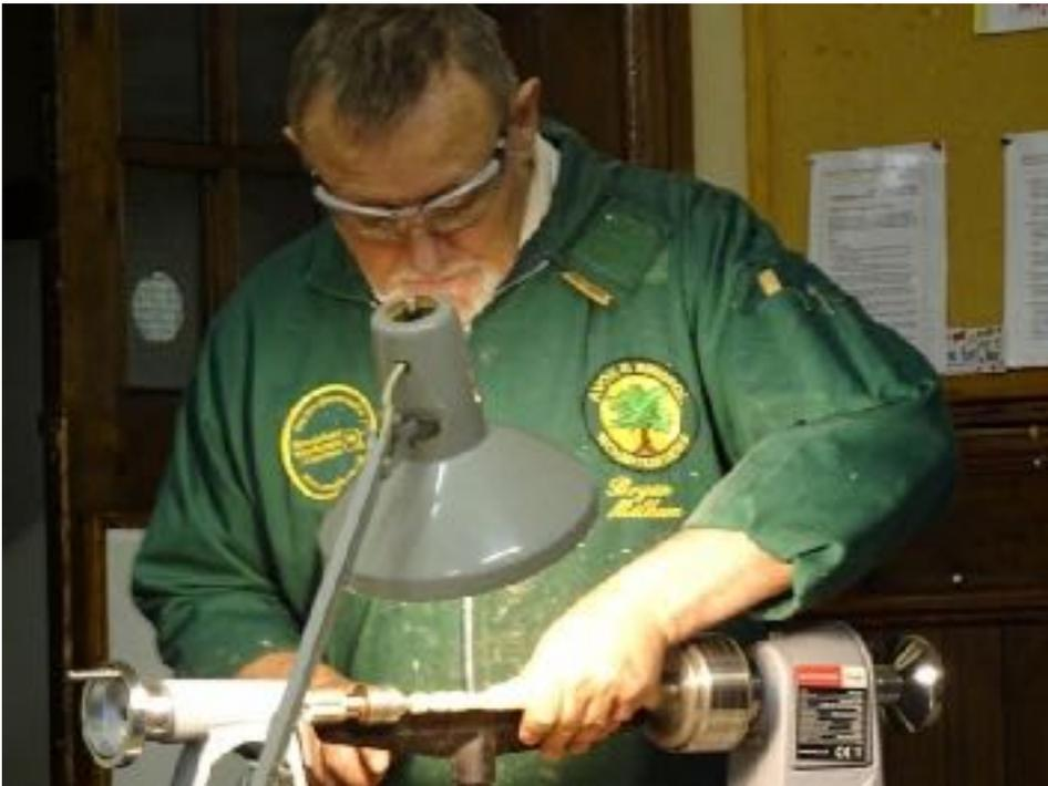
**Top Tip 1** - when using the skew, mark a line down the middle of the skew and then always cut below the centre line.
