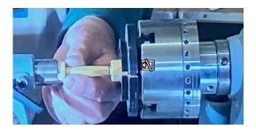
The shape of the tailstock and headstock parts of the press are as shown in the photos below, noting that the tailstock part is tapered but not to a tight fit as it is held in place against the shoulder ...
