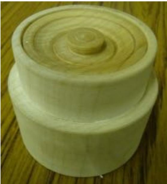
Finally, another jamb chuck was made to hold the base while the bottom of the base was cleaned up and made slightly concave so that the box sits firmly on a solid surface.
