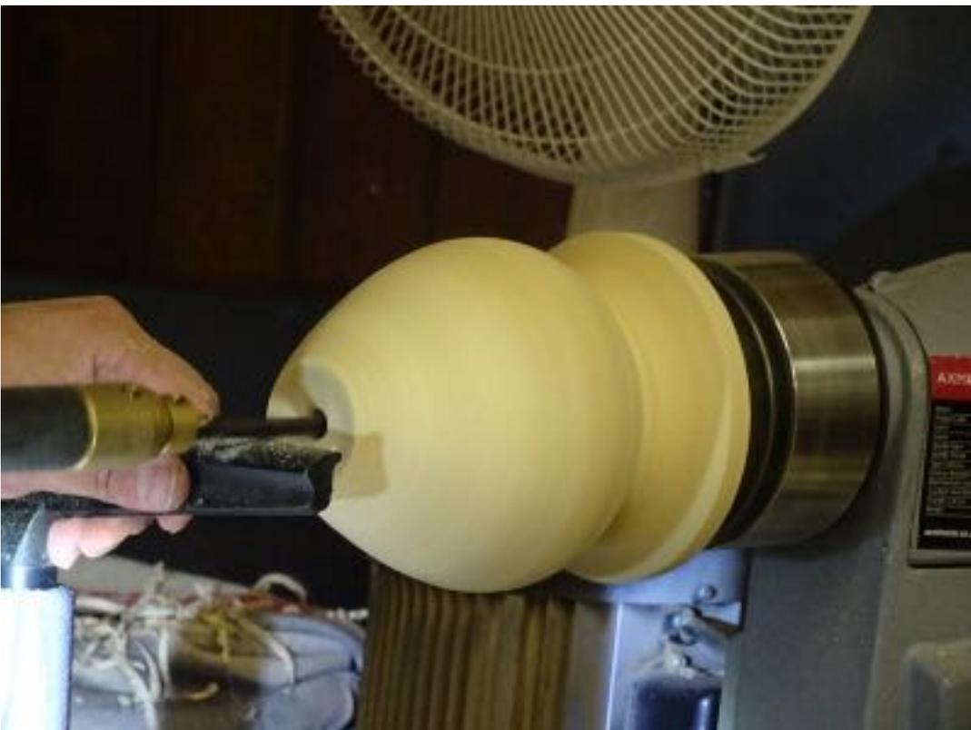
As normal, the blank was turned to round, a spigot formed and the piece remounted and the front face cleaned and squared off.
