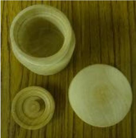
The size of the box was much reduced from the genuine Japanese tea box, purely to demonstrate the techniques involved and was all turned from a single spindle of seasoned sycamore. The process results in a box where the grain of the main lid and bottom do not match, which is not an issue, as the genuine boxes would normally be lacquered.
