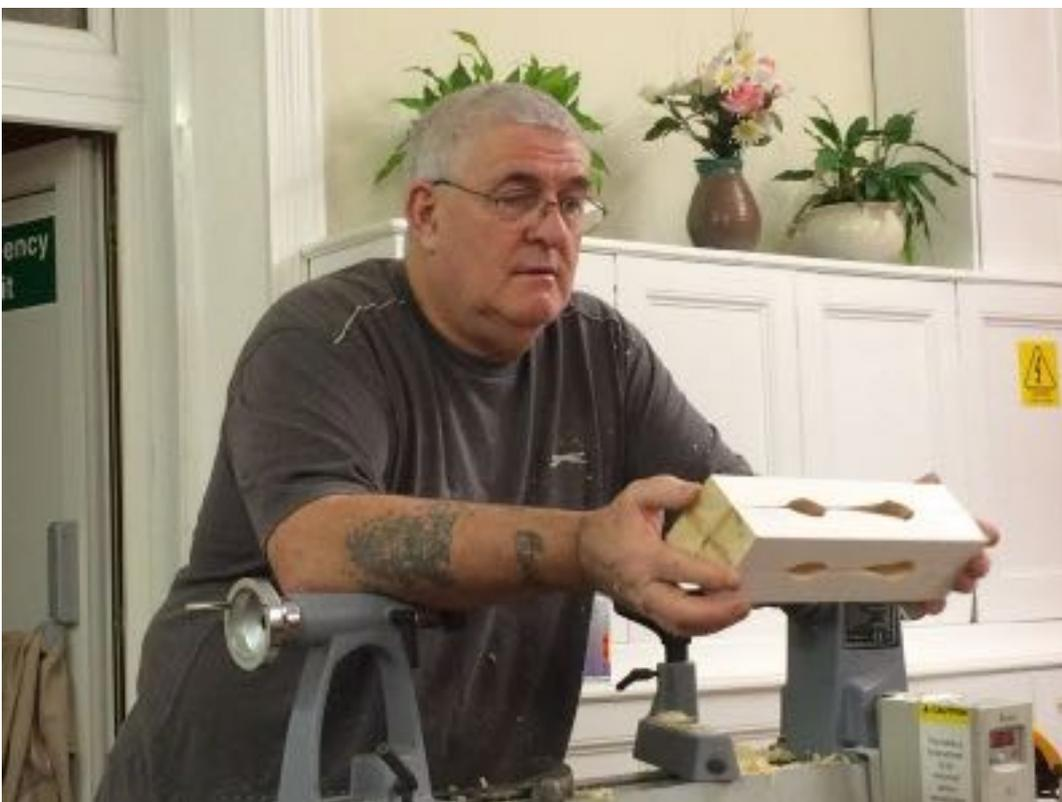
The new composite spindle was now remounted in the lathe and for safety a spigot was cut on one end and then the piece turned to round ...
