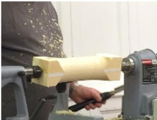
The block was mounted on the lathe using a stepcentre in the headstock to assist keeping the 4 pieces together and a cup centre in the tailstock. The piece was then turned to round whilst leaving of the order of 1 to 2ins of square on the ends to ensure the piece remained intact.
