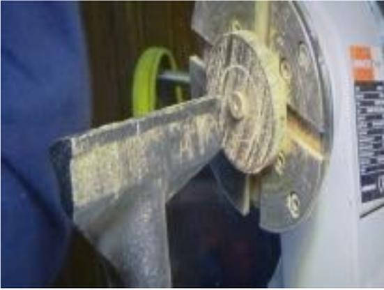
... bringing the tailstock up (not too tight) to support the work whilst the main body was turned to round before locating on the other spigot hole to complete the operation ...
