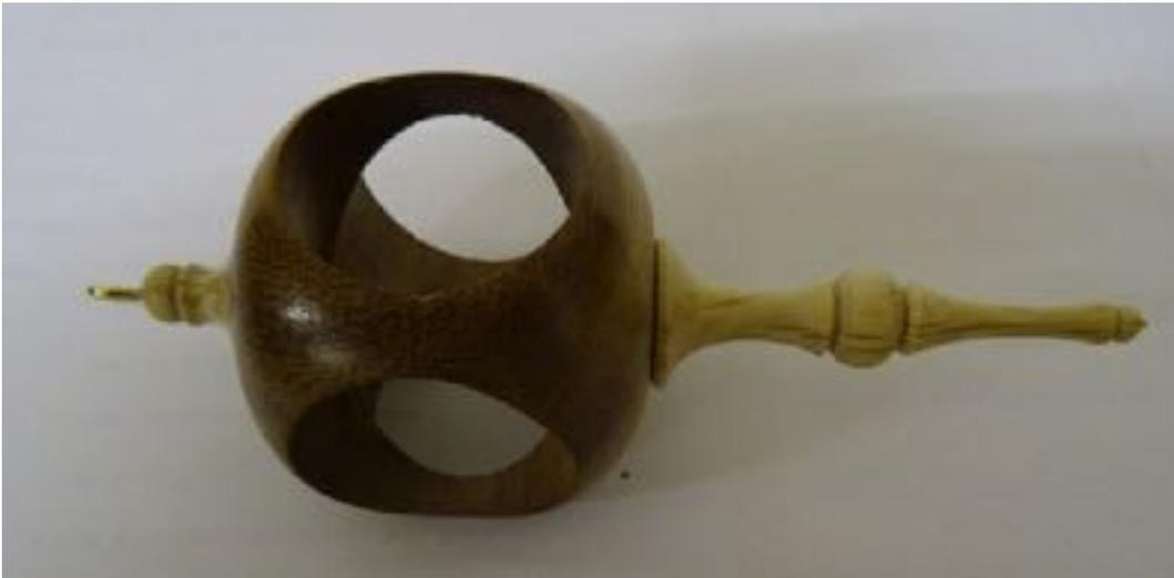
The starting point for the demonstration was the main body which was an **exact** cube of mahogany type wood. Firstly, two opposite sides were drilled to receive the finials making sure that the holes did not penetrate into the middle of the turned body.
