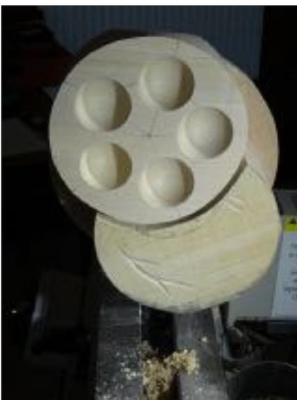
To mount the bowl blank the jig baseplate was mounted in the headstock and then with one of the bowl centre points precisely aligned with a sharp pointed revolving centre in the tailstock, the bowl blank could be held in place in place with a 2 or 3 screws.
