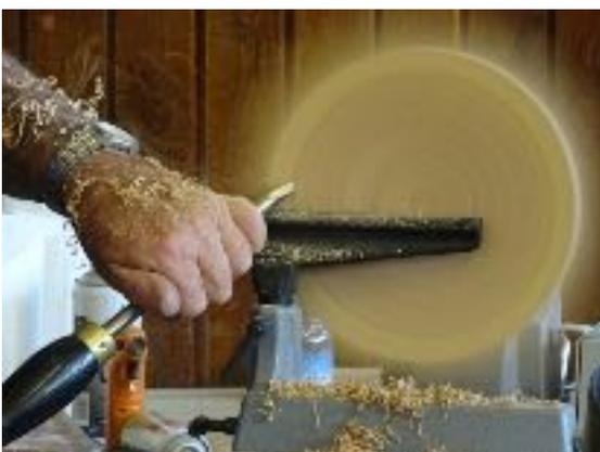
Having turned a spigot of the optimum size for the chuck the bottom of the platter was then finished with a scraper and then sanded from 120 grit down to 400 grit.
