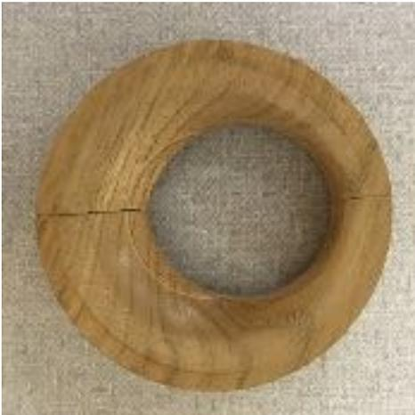
To complete Jig#1 the jig is sawn in half on the bandsaw and then reconnected together using elastic bands in the 2 grooves on the outer edge.
