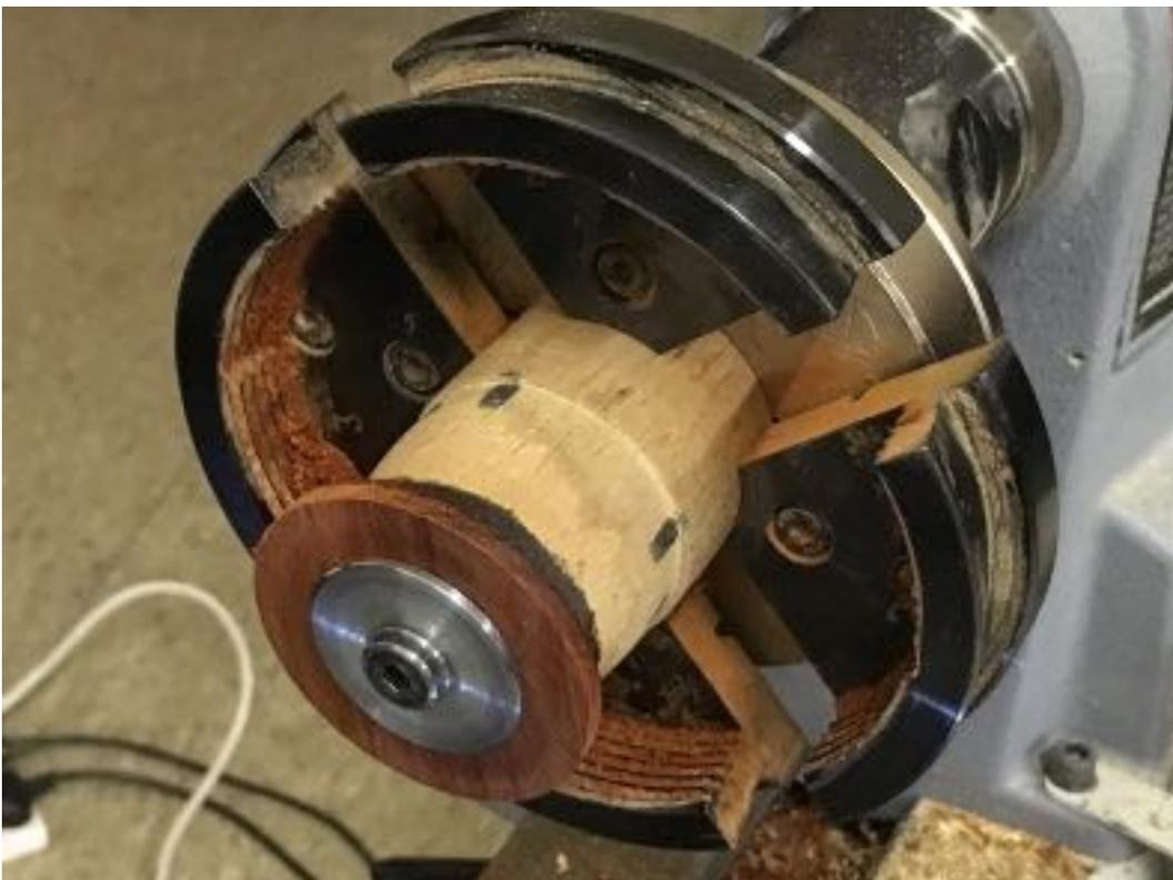
A bolt, penny washer, the pendant, washer made from mouse mat type material, and a nut glued into the spindle appropriately sized to fit the chuck jaws. Note that it is a good idea to glue the nut into the rear end of the jig to prevent it pulling out.
