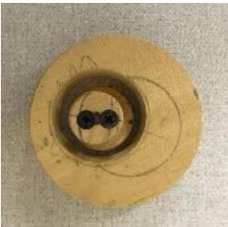
The picture shows Jig#1 with the offcentre hole now separating it from the piece which was attaching it to the original chuck mounted blank.
