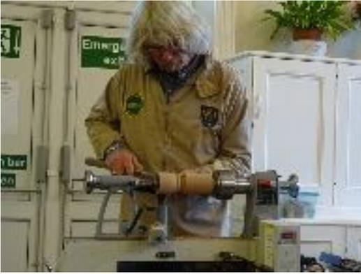
Holding the bowl in the tailstock with a modified revolving centre with a soft nose, Pete started to shape the stem of the goblet. As a diversion, he showed us how to create captive rings. Firstly, using a thin parting tool to create the correct ring thickness, Pete then cut the rings off using his homemade ground to a point allen key tool.
