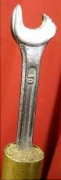
Because the creation of these spigots is used a lot, a quick and consistent method of creating them was required and Pete had again devised his own tool by modifying spanners of the correct size, in this case 8mm. It was then just a matter of drilling an 8mm hole in the stem to ensure a perfect fit without having to constantly resort to calipers.
