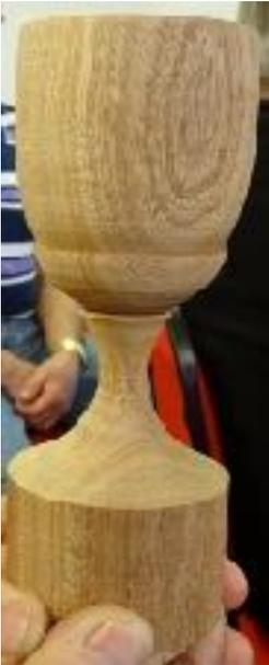
For the demo the rings were then removed and the stem shape completed noting that whilst the relative shape and form of the bowl and stem may look OK when held horizontally on the lathe, it is as well to remove from the lathe from time to time as the vertical look of the piece may be different to the eye, and it is in the vertical position that the finished piece will be used, although with overuse it may well end up horizontal again!
