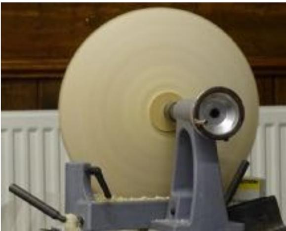
Mounting the blank in the chuck the first task was to level and finish the top flat surface using a pull cut with a bowl gouge, then sharp scraper and finally with abrasive after turning the lathe speed down to reduce heat.
