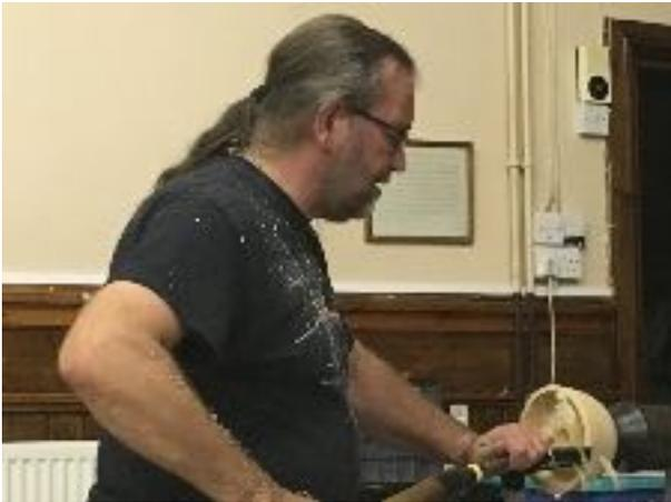
With the inside complete the work was mounted on a friction drive to complete the shaping of the foot.
