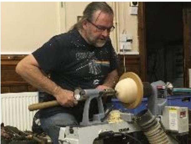
**Top Tip 5** - Look at the Tormek sharpening method for sharpening a parting tool to get clean side cuts
