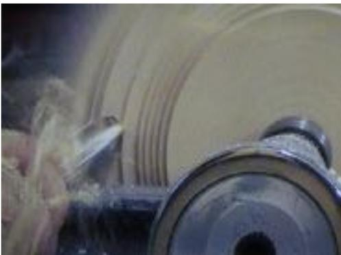
**Top Tip 2** - as ever when turning a square edged piece be aware of the position of the hands and keep well away from the revolving wings.
