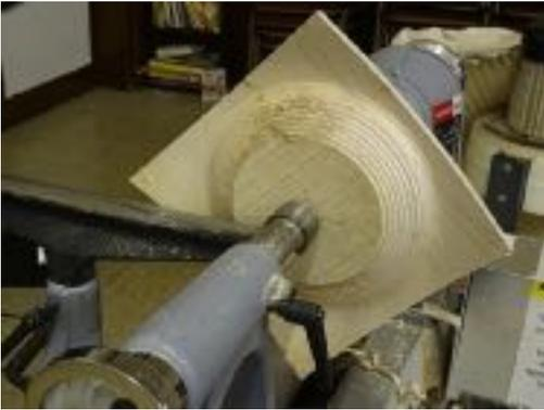
To create the lid, the smaller block was held by a revolving point and ring centre and gripped against the opened out chuck jaws **without using a faceplate etc** which all looked a bit hairy but as the small piece was tightly held there was no problem and was sufficient to enable a spigot to be turned to fit into the bowl recess.
