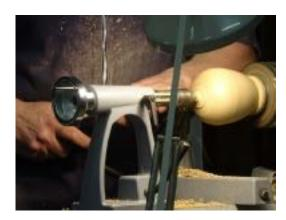
Mount the lid and hollow out, initially making a hole right through to form the vessel opening. Continue the hollow out up to the registration mark and then use a skew to create an almost parallel side (tapered inwards slightly) until the base fits snugly bearing in mind that the lid and base will eventually be glued together once the hollowing of both baser and lid has been completed.
