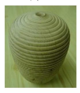
Using a standard box method ... block held in 4-prong drive, turn to round, spigot on each end, shape the general form, 6mm parting tool at lid/base join and then again to increase rebate to 9mm, and finally a 3mm parting tool to separate the lid and base leaving a registration mark on the lid to highlight the max width of the base spigot.
