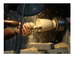
The inside of the hollow form was finished with a scraper.
