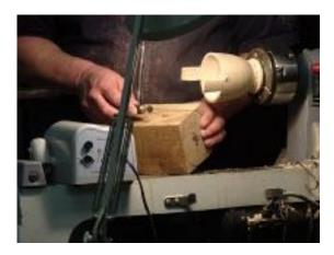
The bucket was now reverse mounted in the chuck using a jam chuck and router mat so that the base could be finished off using a spindle gouge and skew to create an indented base which was finally sanded smooth.
