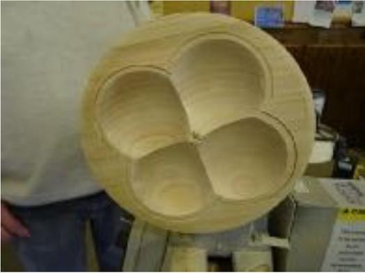
The faceplate was remounted on the centre of the blank. Note that the 5 holes in the faceplate are not necessarily equidistant apart so either mark the position of the faceplate when first used, or rotate the faceplate until the holes match with the originals, or fix using new screw holes.
