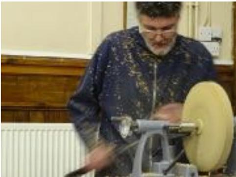
Having shaped the bottom of the platter a scraper was used to create a smooth surface, sanding being left until the top of the platter had been shaped.
