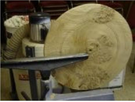
The outer edge was then shaped before cutting in, starting at the bead, to complete the shape of the outer 1/3.
