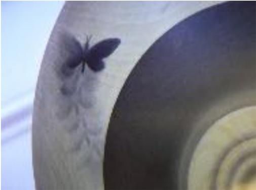
**Top Tip 6** - having completed the outside design work, finish with a "fog" of lacquer rather than oil as the latter will go yellowy over time
